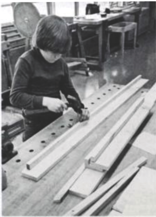
After Starr rips the sides for the hockey board on his radial-arm saw, he has the kids nail and glue ledger strips to the bottom edges, left. Children should be reminded not to put nails too close to the ends of the boards, to avoid sawing through them when the sides are mitered. At first, mitering is confusing for children, so Starr bangs a mitered mirror frame on the wall as a teaching aid. Above, a fifth-grader saws a miter on one end of a board hockey frame.
