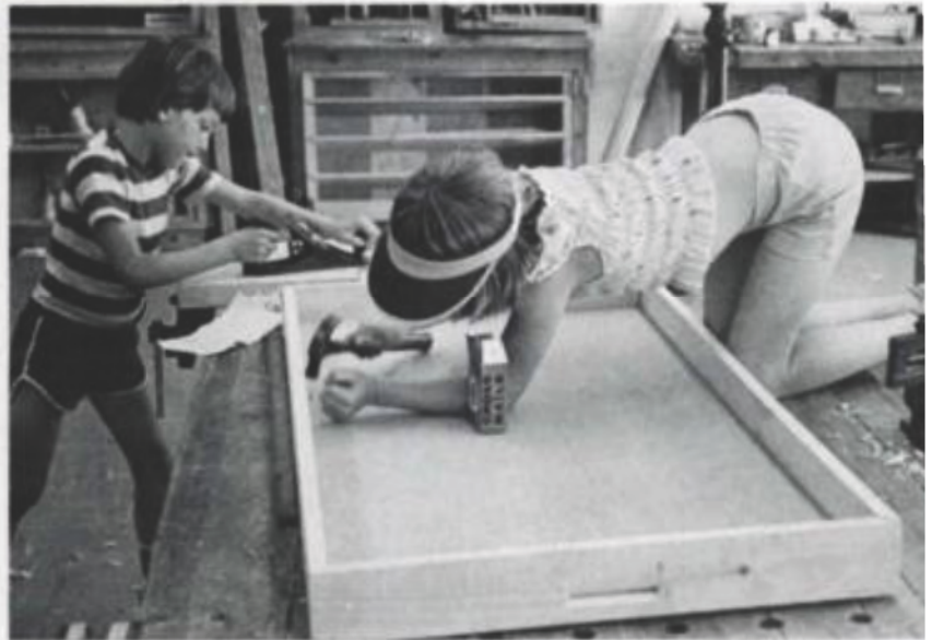
After Starr rips the sides for the hockey board on his radial-arm saw, he has the kids nail and glue ledger strips to the bottom edges, left. Children should be reminded not to put nails too close to the ends of the boards, to avoid sawing through them when the sides are mitered. At first, mitering is confusing for children, so Starr bangs a mitered mirror frame on the wall as a teaching aid. Above, a fifth-grader saws a miter on one end of a board hockey frame.
