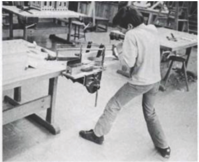
After Starr rips the sides for the hockey board on his radial-arm saw, he has the kids nail and glue ledger strips to the bottom edges, left. Children should be reminded not to put nails too close to the ends of the boards, to avoid sawing through them when the sides are mitered. At first, mitering is confusing for children, so Starr bangs a mitered mirror frame on the wall as a teaching aid. Above, a fifth-grader saws a miter on one end of a board hockey frame.
