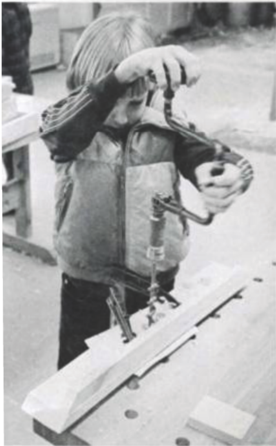
Making a board hockey game gives children a chance to learn several basic skills: sawing, boring, chiseling and nailing. Above, a second-grader uses an auger to bog the waste out of one of the hockey board's goal openings. He'll finish the job with a chisel and a file. Above right, a student nails the plywood bottom into the hockey board. The completed board, right, will be given a coat of shellac, followed by wax for a fast-playing surface.
